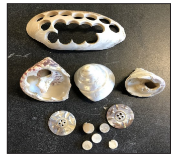
Top to bottom: A mussel with holes from punched-out blanks; white abalone shells; red and white trochus; two finished buttons and five unfinished blanks. (Credit: Kristen Goodhue/SERC)
